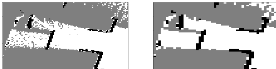
Figure 3. An example of max pooling of the built map. Gray denotes an unknown area, black denotes obstacle cells, and white denotes free space cells.
