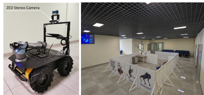
Figure 7. Robot platform based on the Clearpath Husky chassis with a ZED camera ( left ). We used it to evaluate our results in a real-world scene ( right ).
