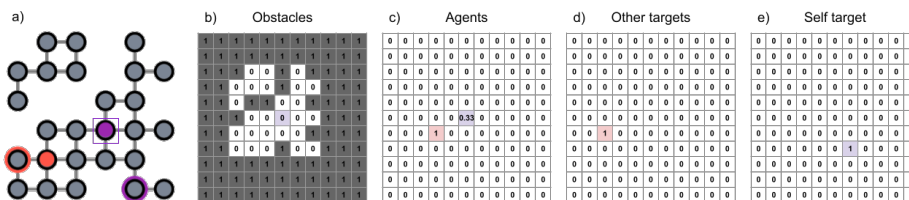
Fig. 3. An example of an observation matrix for a purple agent. In all observation cells, 1 means that there is an object (obstacle, agent, or goal) in this cell and 0 otherwise. a) Environment state. The agent for which the observation is shown is highlighted; b) Obstacle map. The central cell corresponds to the position of the agent, in this map the objects are obstacles; c) Agents map. In this map, the objects are agents; d) Other agents' goals map. In this map, the objects are the goals of other agents; e) Goal map. In this map, the object is the self-goal of the agent.
