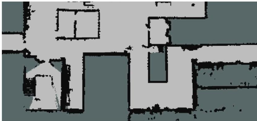
Fig. 17. Occupancy Grid map of the environment for real robot experiments. Artificial narrow passages may be seen in the top left area.
