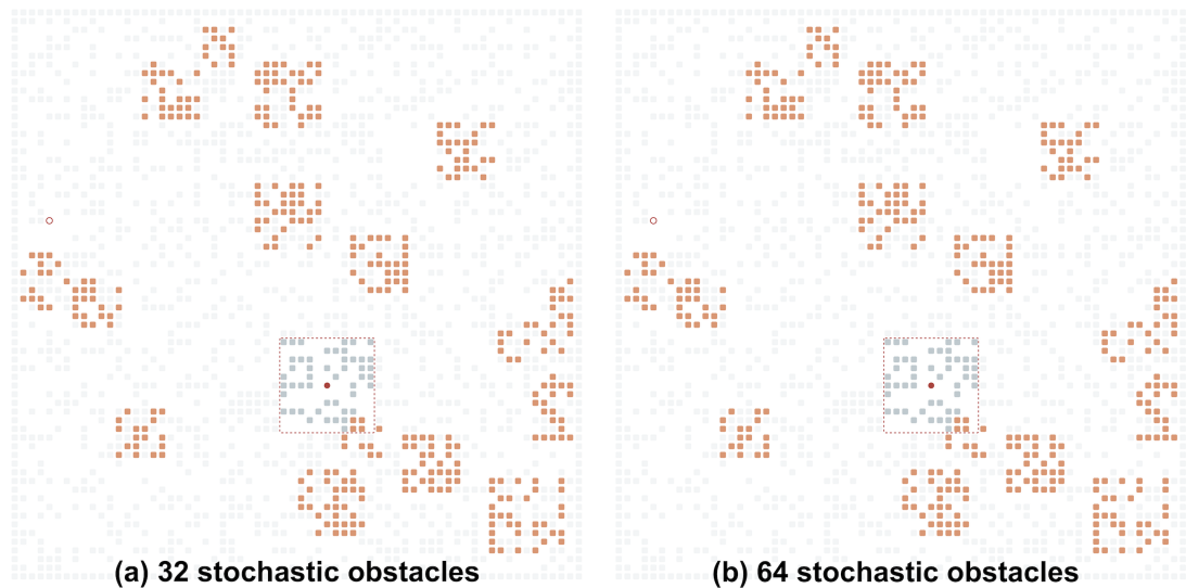
Figure 2. Examples of the grid environments with different numbers of the stochastic obstacles (shown in orange). Undiscovered static obstacles are transparent. The agent’s field of view is shown by the red square.
