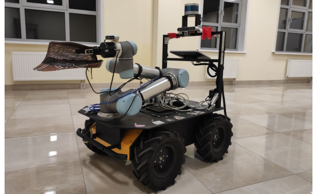
Fig. 6. Husky mobile manipulator transporting a hat. A footprint with an outstretched manipulator is valid for this task.
