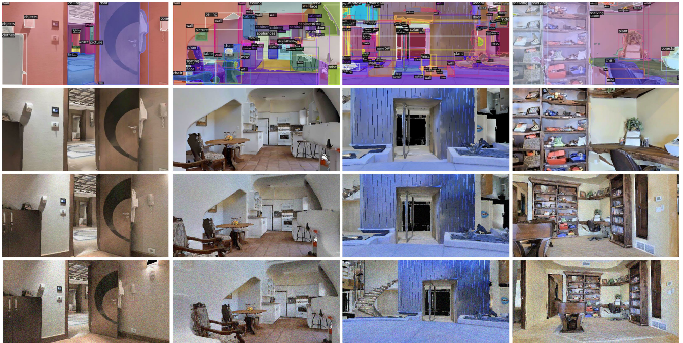
FIGURE 2. Examples of images from HISNav Dataset with three levels of noise: the first row contains visualization of ground truth segmentation, second row demonstrates images without noise, the third row includes images with light Gaussian noise ( mean = 0, \sigma = 1, intensity = 0.05 ), the bottom row contains images with strong Gaussian noise ( mean = 0, \sigma = 1, intensity = 0.1 ).
