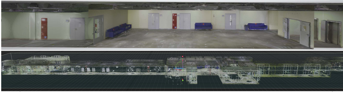
FIGURE 11. The bottom image is how the point cloud looks before texturing. The upper image is after texturing at RealityCapture.
