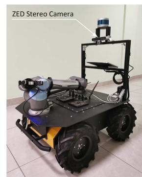
FIGURE 1. Ground robot platform based on the clearpath husky chassis with a ZED camera. We used it to evaluate our results in real-world scenarios.
