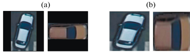
Fig. 8. Two types of squaring cut-out images with vehicles: (a) filling an empty area of the image with zeros (padded images), (b) stretching the image (stretched images).
